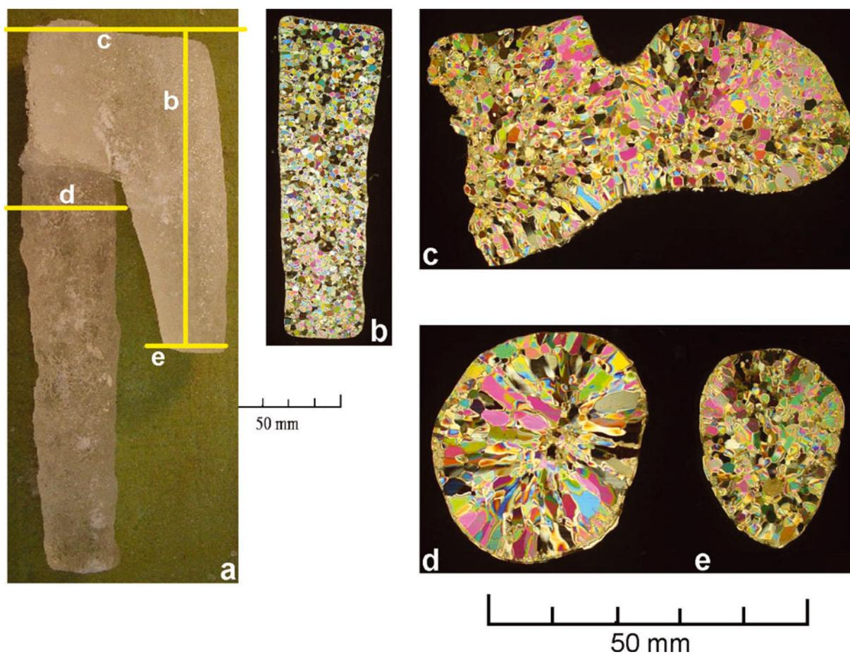
**Fig. 4.** Photographs of spray-ice sample C obtained on 31 January 2008: (a) external view; (b) vertical thin section of the right branch; and (c–e) horizontal thin sections (marked by yellow lines in (a)) at various depths. The left branch was ~250 mm long.
